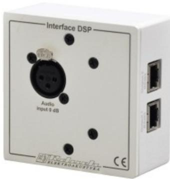
DSP interface is a device used for communication between the PC and the ACML columns. It is also used to transmit the 0dB signal to the ACML columns. Communication is via the serial interface (USB-USB cable).
