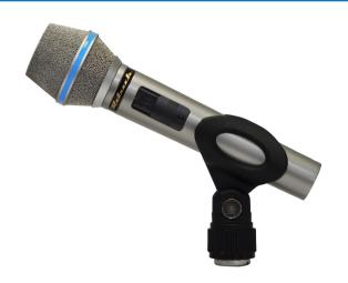
CMSN condenser microphone with a supercardioid frequency response, very good front-to-rear attenuation, low noise, guarantees perfect crystal sound throughout the entire acoustic spectrum. The CMSN microphone uses a gold-plated diaphragm with a diameter of 18 mm, installed in a housing made of brass, galvanized with matt nickel or powder coated in black. The CMSN microphone is equipped with a sliding switch. The accessories include a windscreen, microphone holder and case.
