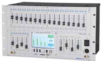
Modern mixer equipped into DSP signaling processor which allows precise correction of sound characteristic in buildings with very difficult acoustic conditions. Mixer activates only those microphones that are being used at the moment, which eliminates the influence of the surrounding sounds coming from unnecessarly opened microphone channels (one of the programming option).
